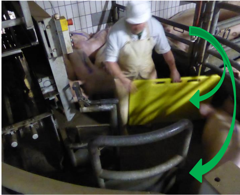
The corral shaped raceway had two entrances to the single file chute, so the pigs have a choice.
